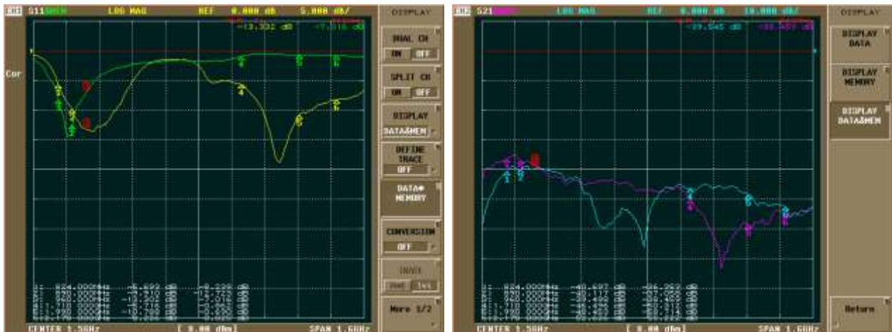
Figure 53: |S_{11}| and |S_{21}| comparison of a 900 MHz tuned half wavelength dipole and a penta-band internal antenna
