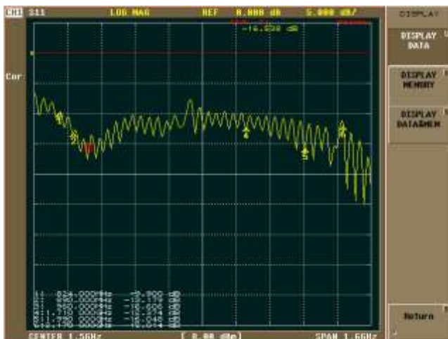
Figure 52: |S_{11}| sample measurement of a wideband antenna
