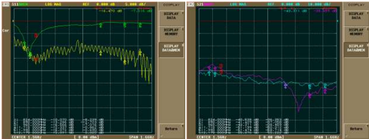
Figure 57: |S_{11}| and |S_{21}| comparison between a 900 MHz tuned half wavelength dipole (green/purple) and a wideband commercial antenna (yellow/cyan)
