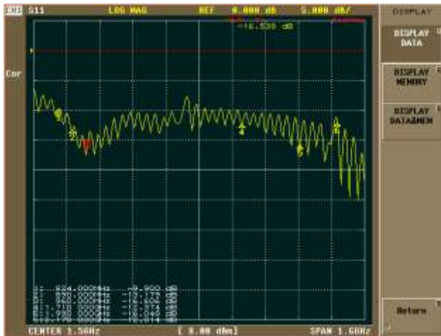
Figure 55: |S_{11}| sample measurement of a wideband antenna
