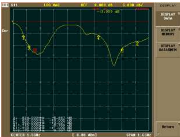
Figure 54: |S_{11}| sample measurement of a penta-band antenna that covers in a small form factor the 4 GSM bands (850 MHz, 900 MHz, 1800 MHz and 1900 MHz) and the UMTS Band I
