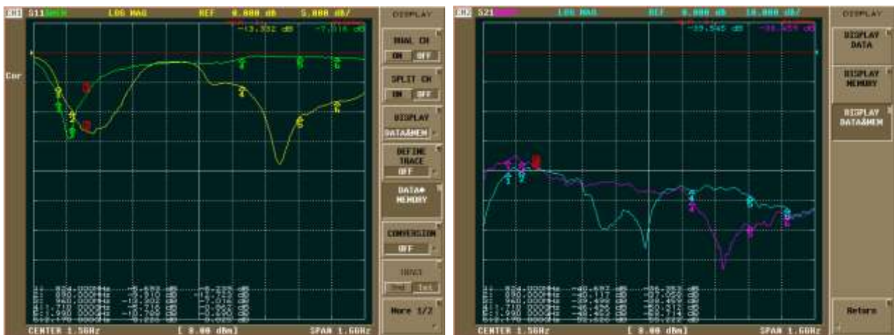
Figure 56: |S_{11}| and |S_{21}| comparison between a 900 MHz tuned half wavelength dipole (green/purple) and a penta-band internal antenna (yellow/cyan)
